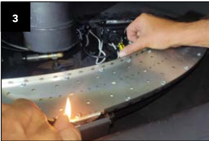
3 Hold the valve down and use a lighter to check for gas at the pilot. Air will initially escape.
